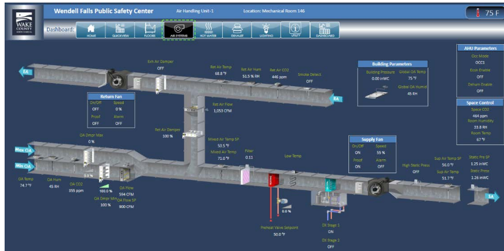
Figure 7: AHU Graphic, Example 1
