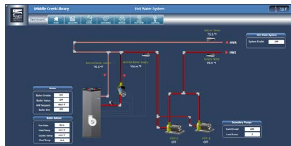
Figure 17: Boiler Plant Graphic, Example 1
