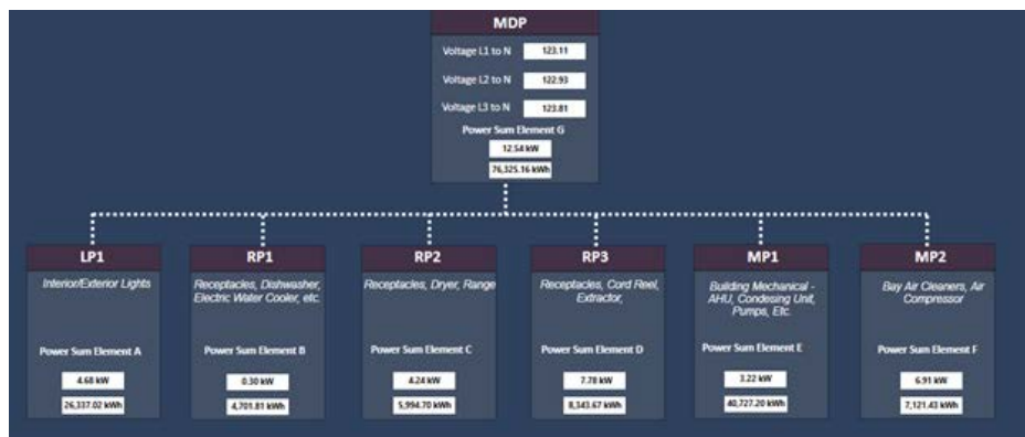
Figure 22: Power Meter - Riser/Tree Example
