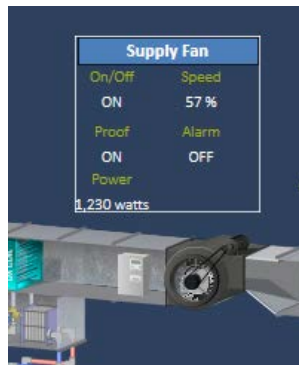
Figure 15: VFD points in Equipment Graphic
